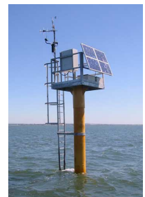
Visibility sensor on Met station in sea
