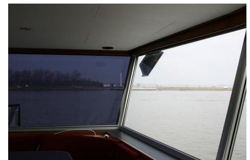
Sunblinds installed at a moter vessel
