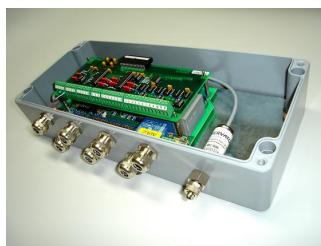
Barometric pressure sensor in OMC-183
